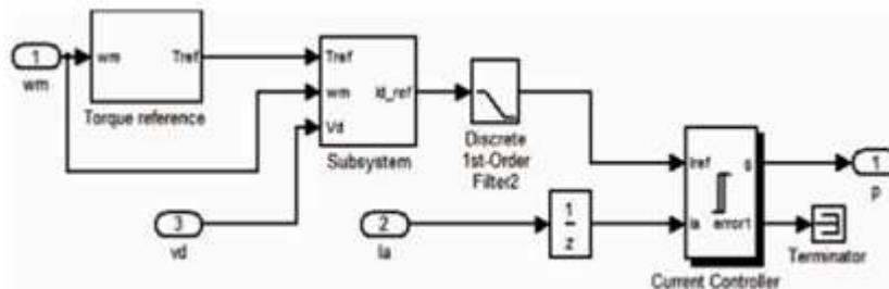
**Figure 3: Sub-System Implementation of MPPT control for Wind Power System.**
