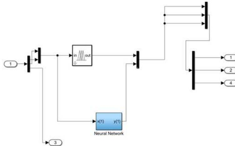
**Figure 6: Block Diagram of FNN Based Controller of VSI.**
