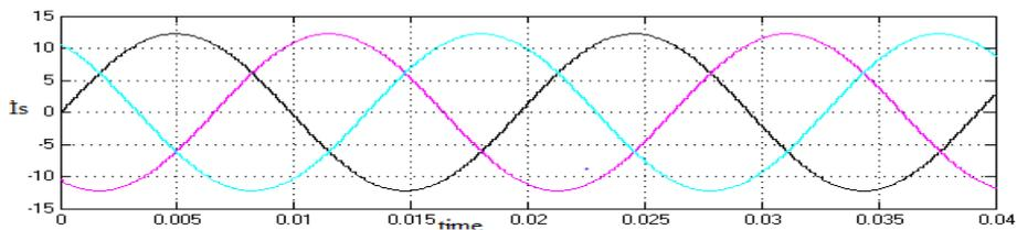
Figure 15: VSI Output Current Source.
