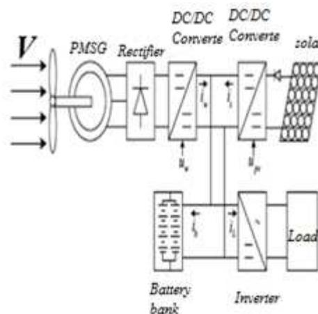
**Figure 1: Block Diagram of PV-Wind Hybrid System.**
