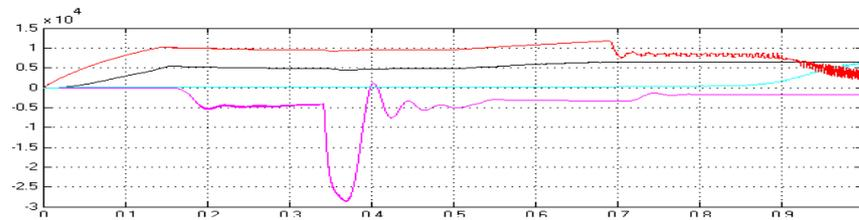
Figure 10: Power Generation of the Hybrid System under Varying Wind Speed and Irradiation.
